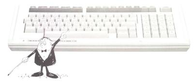
Alpha-Numeric Keyboard: typewriter keyset, numeric keypad, user-defined soft keys, display and system control keys.
