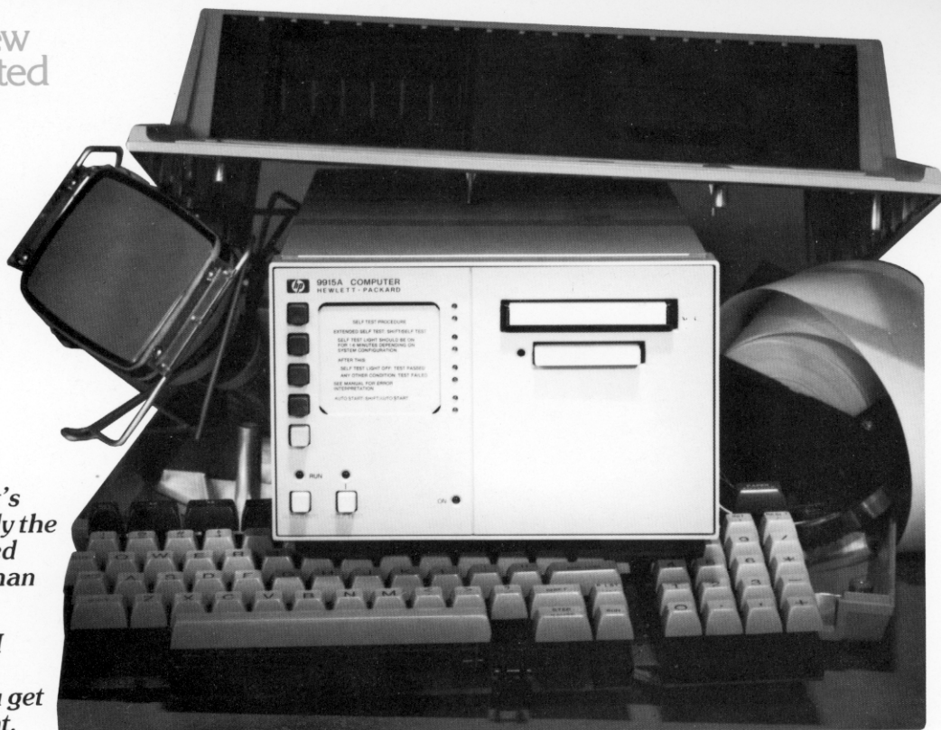
The heart of an HP-85 Desktop Computer in a new, industrial package.
